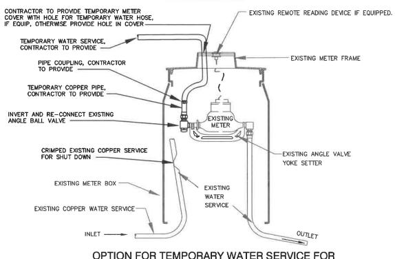
OPTION FOR TEMPORARY WATER SERVICE FOR **OUTSIDE METER SETTING**
