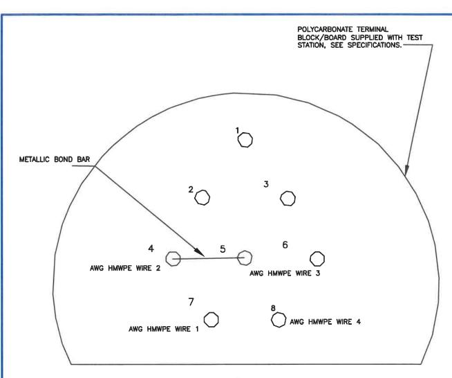
TERMINAL #4 - AWG HMWPE WIRE 2 FROM WATER PIPE 1
